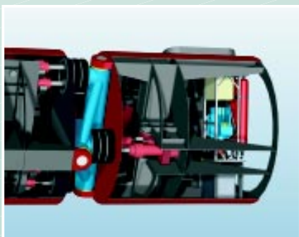
Cross-section of Pelamis Joint Sections with hydraulic rams and Hydraulic Power Pack
